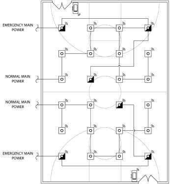
Wiring shown assumes emergency fixtures ordered with integral UL924 dimming bypass module. Please see fixture spec sheet for details on ordering options.
