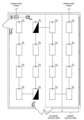
Wiring shown assumes emergency fixtures ordered with integral battery backup. Please see fixture spec sheet for details on ordering options.
