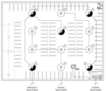
Wiring shown assumes emergency fixtures ordered with integral UL924 dimming bypass module. Please see fixture spec sheet for details on ordering options.
