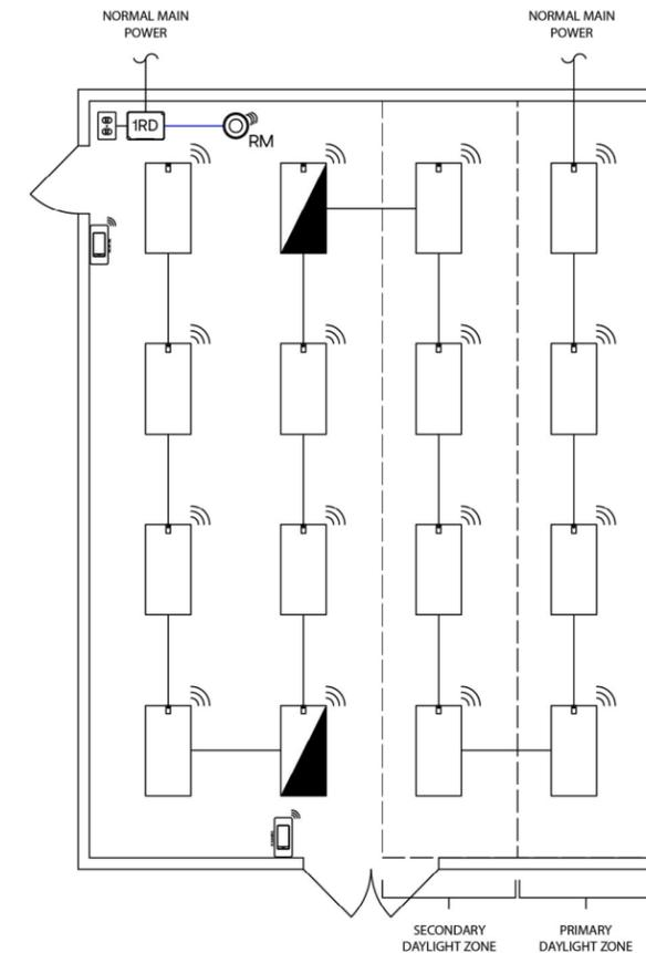
Wiring shown assumes emergency fixtures ordered with integral battery backup. Please see fixture spec sheet for details on ordering options.
