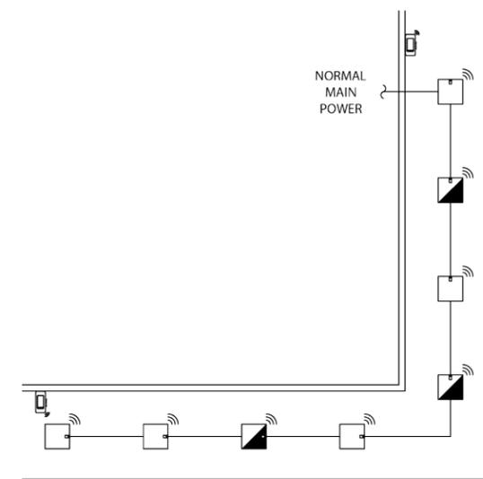
Wiring shown assumes emergency fixtures ordered with integral battery backup. Please see fixture spec sheet for details on ordering options.
