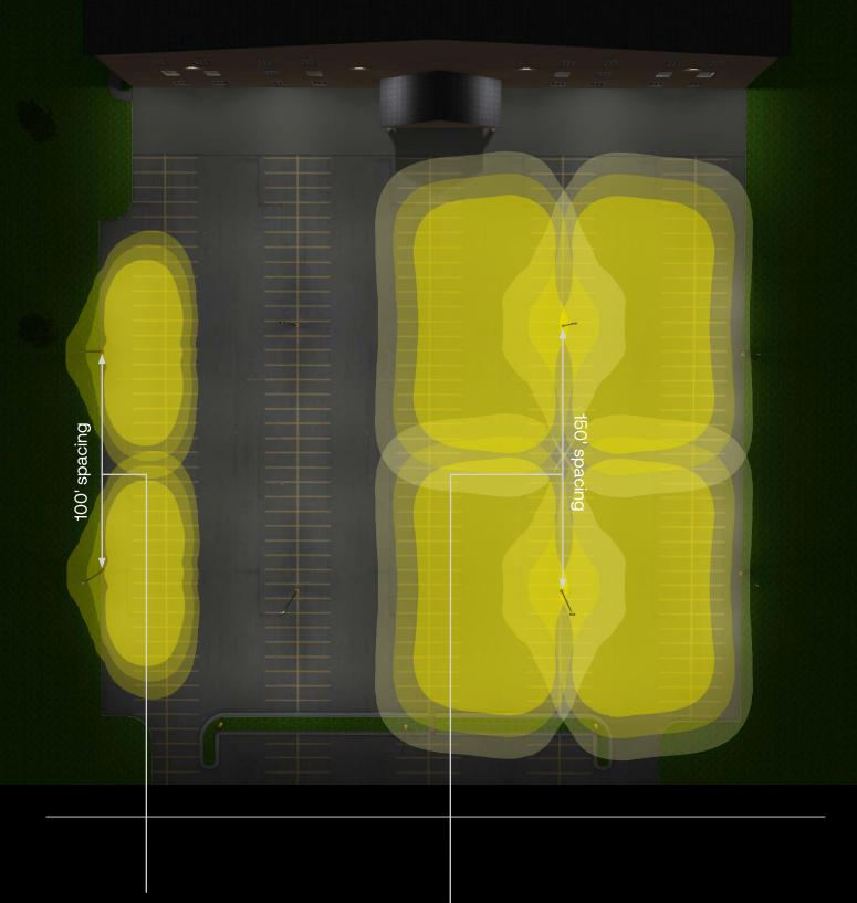
The 135W Sling replaces 400W legacy luminaires and can be seen here on 25ft poles. The Type III distribution provides great spacing between poles and minimal backlight.
