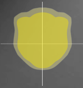
TYPICAL AREA/SITE LUMINAIRE 20–30% backlight
