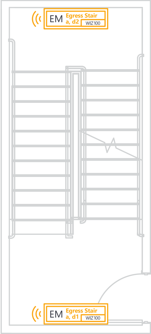
Egress Stairwell Daintree One 5-WIZ100-Integrated fixture control with daylight and occupancy
