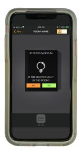
**Devices will identify themselves** by blinking. The app identifies fixtures by proximity. Simply move closer to fixtures that need to be programmed within the zone or aisle.
