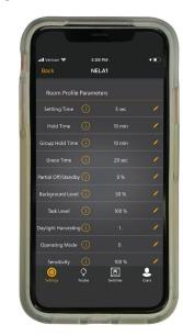
**Create profiles** ensuring zones and aisles function consistently with the determined sequence of operation based on user need and local energy code requirements.
