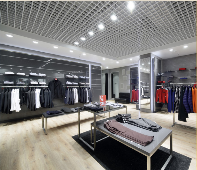
Alternative shallow aperture solutions create greater ceiling glare
