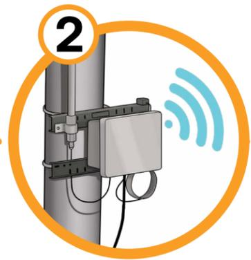
The gateway connects nodes to the Central Management System through a standard TCP-IP interface. Optional wireline connectivity available.
