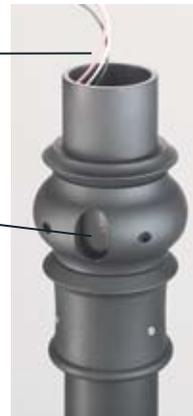
The PCA Photocell Module is an innovative way of overcoming problems with photocells that cycle the lamp because of unwanted light sources in the environment. The PCA Photocell Modules are rotatable 360 degrees, so the photocell can be aimed away from light sources. The Photocell Module accepts a standard, twist lock photocell. The module has a acrylic window to protect the photocell from the elements and premature failure. The photocell is also shielded from light emissions from the fixture.
