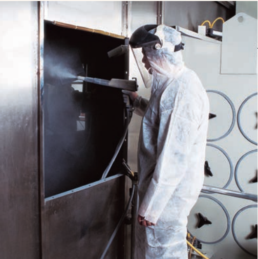
Kim's TGIC powdercoat finish is applied electrostatically for added durability
