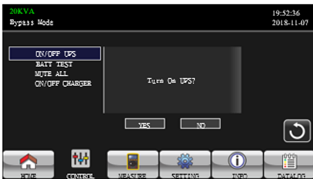
Turn ON UPS
