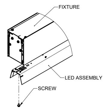
REMOVE LED REFLECTOR MODULE(S) BY REMOVING (2) 8-32 MACHINE SCREWS. ALLOW MODULES TO HANG ON TETHERS.
