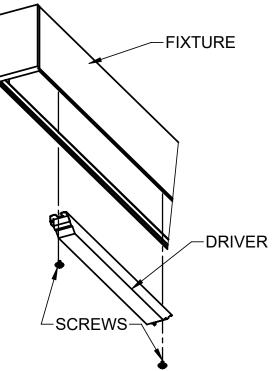
BEFORE REMOVING DRIVER SEE STEPS 8 AND 9 FOR LENS AND LED TRAY REMOVAL. REMOVE THE (2) SCREWS AS SHOWN AND REMOVE DRIVER.
