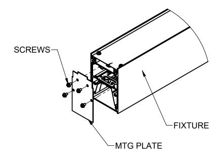
TO REMOVE END CAP MOUNTING PLATE REMOVE THE 6-32 MACHINE SCREWS SHOWN ABOVE.
