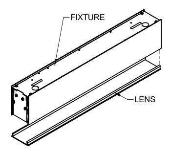
TO REMOVE, PULL LENS DOWN TO DISENGAGE LENS FROM FIXTURE.FOR INDIVIDUAL FIXTURE, REMOVE ONE END CAP PER STEP 7.
