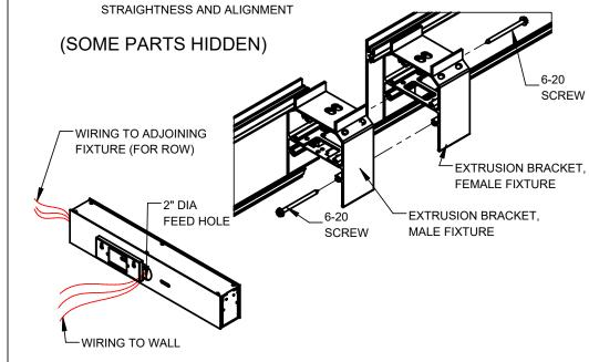
BRING ELECTRICAL FEED INTO FIXTURE WIREWAY AND MAKE WIRING CONNECTIONS. FOR ROW, WIRING CAN BE BROUGHT THROUGH ENDS AT EACH JOINT.
