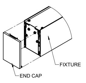
REMOVE THE END CAP BY PULLING END CAP TO DISENGAGE MAGNETS AND LIFT UP TO DISENGAGE FROM TAB ON END CAP PLATE.
