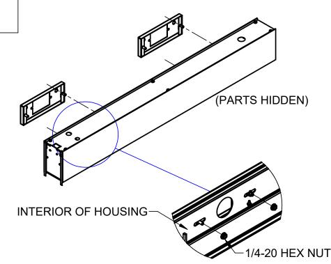
LIFT AND MOUNT FIXTURE ONTO WALL BRACKET(S). USE 1/4-20 HEXHEAD NUTS PROVIDED. IF INSTALLING ROW, DO SO FOR 1ST FIXTURE ONLY.
