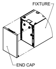
REMOVE THE END CAP ASSEMBLIES BY PULLING END CAP TO DISENGAGE MAGNETS AND LIFT UP TO DISENGAGE FROM TAB ON END CAP PLATE.
