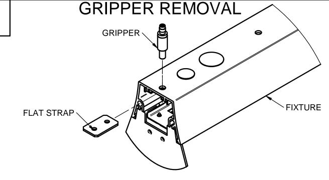
TO REMOVE GRIPPER, COMPLETELY UN-SCREW CABLE GRIPPER UNTIL BOTTOM THREADS OF CABLE GRIPPER RELEASE FROM FLAT STRAP. SLIDE OUT FLAT STRAP FROM REST AREA ON EXTRUSION TO REMOVE FLAT STRAP. REPEAT FOR ALL CABLE GRIPPERS ON FIXTURE.
