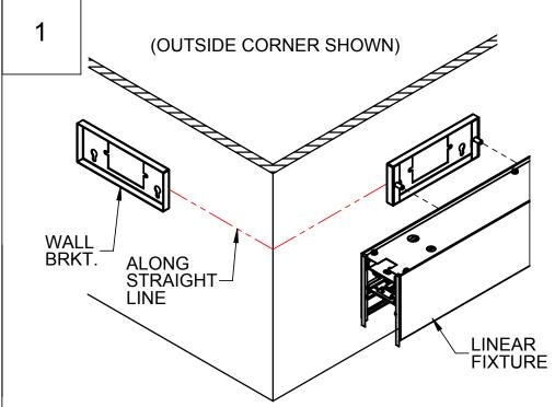
LOCATE THE WALL BRACKETS OF THE LINEAR FIXTURES ADJACENT TO THE CORNER; SEE PLAN VIEW ON PAGE 1 FOR DIMENSIONS. MOUNT LINEAR FIXTURE AT ONE END OF THE CORNER. FOLLOW INSTRUCTION SHEET 510637.
