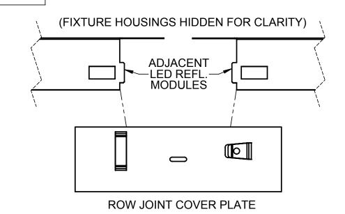
ATTACH ROW JOINT COVER PLATES, AS SHOWN, AT BOTH FIXTURE JOINTS.
