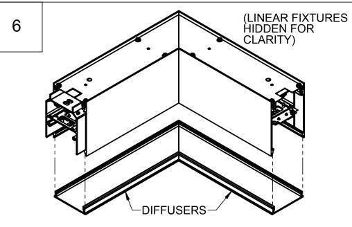
SNAP DIFFUSERS INTO BOTTOM OF HOUSING AS SHOWN. TO REMOVE, INSERT SCREWDRIVER OR FLAT HEAD PRY TOOL INTO SIDE OF HOUSING AND PULL DOWN.
