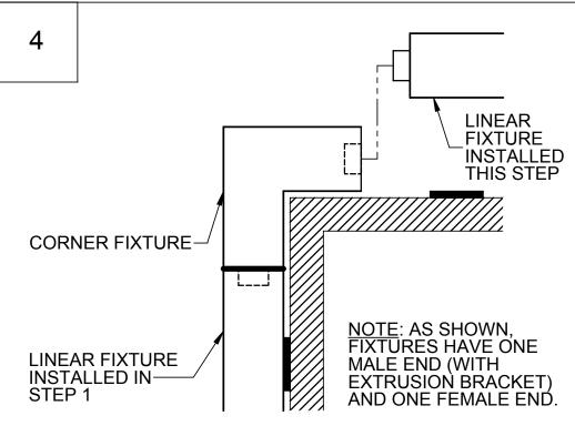
INSTALL LINEAR FIXTURE AT OTHER SIDE OF CORNER AND ATTACH FIXTURES BY FOLLOWING THE PROCEDURE IN STEP 5. MAKE ELECTRICAL CONNECTIONS.
