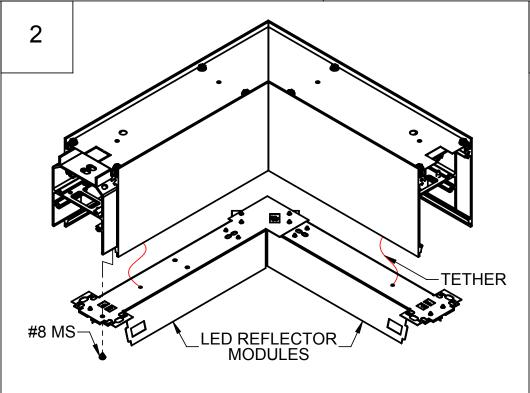
REMOVE LED REFLECTOR MODULES OF CORNER FIXTURE BY REMOVING 8-32 MACHINE SCREWS. ALLOW MODULES TO HANG DOWN ON NYLON TETHERS.
