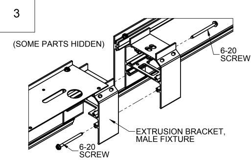
JOIN CORNER FIXTURE WITH MOUNTED LINEAR FIXTURE BY ALIGNING THE EXTRUSION BRACKET AND INSERTING IT INTO THE ADJOINING FIXTURE. SECURE WITH 6-20 X 2" LONG HEX HEAD SCREWS. DO NOT OVERTIGHTEN WITH POWER DRILL. ROUTE BRANCH CIRCUIT WIRING THROUGH FIXTURE JOINT.
