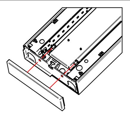
Install end caps by sliding into end headers and attaching with two 10-32 machine screws (provided).
