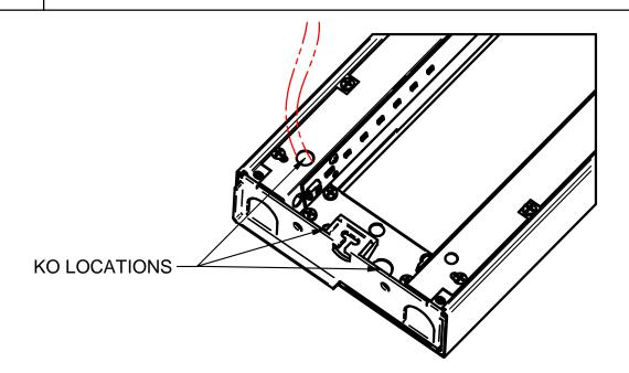
Remove any of the KO on the top LED Module assembly, insert bushing and feed power cord through KO locations near suspension points.
