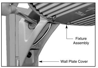
3. Attach fixture assembly to wall plate cover (2 places) using washer and 3/8" bolt. Tighten to 20 ft.-lbs. using 9/16" socket wrench.
