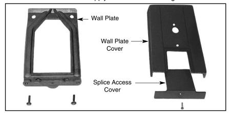
1. Remove splice access cover from wall mount cover and wall mount plate. Apply a continuous bead of silicone sealant compound into the wall plate groove to ensure a proper seal between wall plate and wall.
