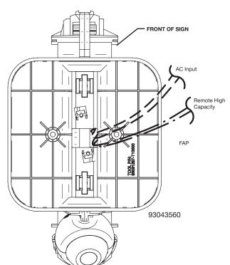
The EVC sign is designed to be wall, ceiling or end mounted. Provide standard and Spectron® equipped signs with single un-switched supply from a 120 or 277VAC branch circuit used for normal lighting in the area to be protected.
