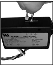
and attach the sensor plugs at the T1 & T2 locations. Do not connect either sensor to the Dim slot.
