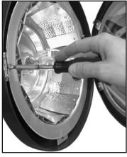
10. Secure reflector with 1/4 turn fastener. Close and secure lens frame.
