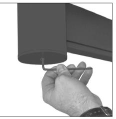
**1.** Install pole and arm cap using a 7/64" allen wrench.
