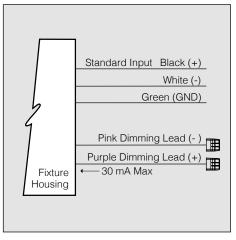
0-10V Dimming: Driver has a 0-10V dimming interface with a dimming range of 10-100%. The driver is compatible with most controls systems including NX Lighting Controls. Note: Not compatible with current sourcing dimmers. Controls compatible via purple and pink dimming leads.
