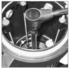
5. Tighten securely to 30 ft/lb using 9/16" socket, 12" extension and ratchet
