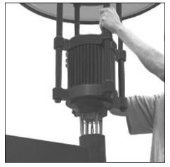
Install fixture assembly on round fitter. Orient fixture relative to mount to provide desired lighting distribution. Tighten securely using 9/16" socket and ratchet with a minimum 12" extension.
