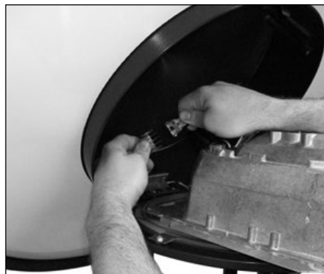
8. Disconnect reflector assembly quick disconnect from fixture quick-disconnect. Remove from fixture.
