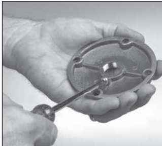
1. Loosen set screw at bottom of mounting device* with Phillips Head screwdriver.
