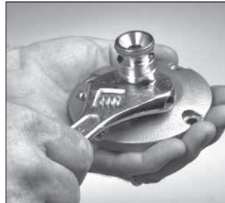
2. Coat coupling threads with a good sealant and tighten coupling onto mounting device*. Re-tighten set screw.
