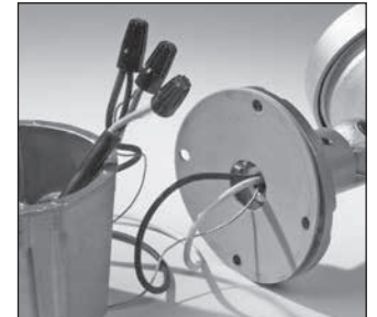
4. white-to-common, black-to-voltage. Screw on Junction box cover, making sure gasket is securely in place.
