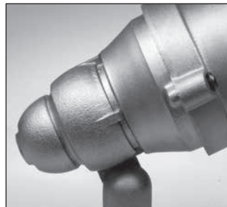
6. After installing lamp, coat shield screw threads with silicone grease and tighten screws progressively. Always install shield with short side down for proper drainage.
