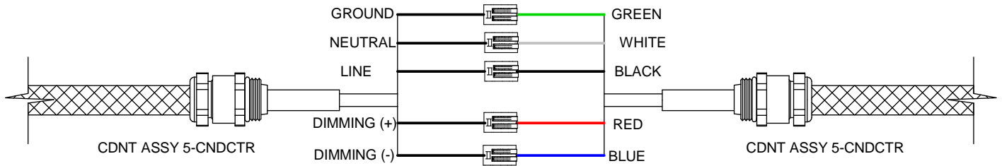
BALLAST COMPARTMENT WIRING
