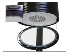
**1.** Open lens frame by loosening self-retaining ¼-20 screws; swing lens frame open until the stop arm prevents further movement.
