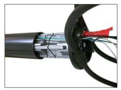
**3.** Lay pole horizontal on padded supports to protect finish. Fish the attached drop leads to the pole hand-hole keeping tension so they aren't caught or pinched. Pick up the fixture and slide the spreader assembly into the pole top. Block the fixture into place. Orient fixture according to light pattern label in reflector. Make sure fixture is square with pole.
