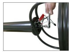
**4.** Tighten the center bolt to 25 footpounds torque. When tight, push the connected wire ends back into the chamber and replace the splice cover.
