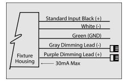
Driver has a 0-10V dimming interface with a dimming range of 10-100%. Is compatible with most control systems including Hubbell Building Automation wiHUBB<sup>™</sup>. Approved dimmers include Lutron Diva AVTV, Lutron Nova NFTV and NTFTV. Note: Not compatible with current sourcing dimmers. Controls compatible via Gray and Purple dimming lead.
