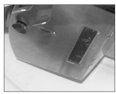
Swing electronic driver assembly into fixture and secure with wing-head screw.
