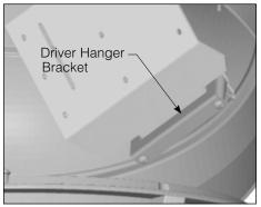
**4.** Connect plug halves between the power lead-in and electronic driver assembly upgrade. Insert tab on electronic driver assembly through slot on driver hanger bracket.
