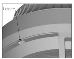
Depress latch to open and gently swing down lens frame assembly for EmitterDeck and electronic driver access.
