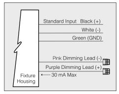
Driver has a 0-10V dimming interface with a dimming range of 10-100%. Is compatible with most control systems. Approved dim-mers include Lutron Diva AVTV, Lutron Nova NFTV and NTFTV. Note: Not compatible with current sourcing dimmers. Controls compatible via Pink and Purple dimming lead.
