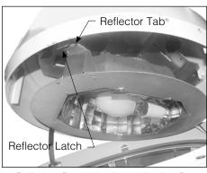
Pull on reflector latch to unhook reflector tab. Lower reflector, disconnect wires, and unlock from the rear hanger to remove the reflector.
