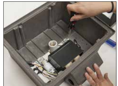
6. Remove (4) Flat Head screws securing ballast tray. Disconnect ballast wiring from line voltage.
