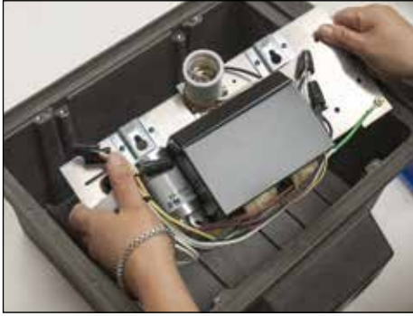
7. Remove ballast assembly.
