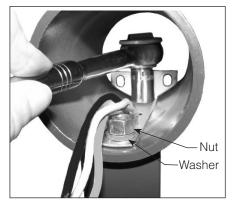
Attach round fitter to arm. Secure with washers and nuts using a 9/16" ratchet wrench.
