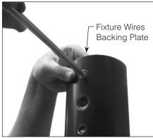
1. Place backing plate inside pole and thread long threaded end of studs ...
