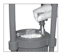
Reinstall driver and secure driver assembly with the two screws provided.
