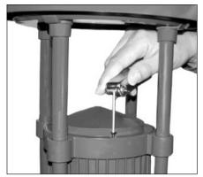
**8.** Remove cover from fixture using a hex wrench.
