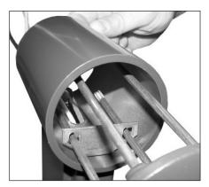
**7.** Install bottom cap with four rods into the two holes in plate alignment.
