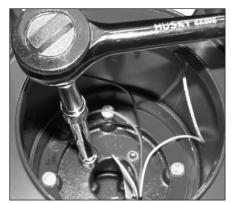
**11.** Orient fixture relative to mount to provide desired lighting distribution. Secure with washers and nuts using a 9/16" ratchet wrench with 10" extension.
