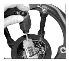
Remove the two screws holding the driver plate in place, and slide driver assembly out.
