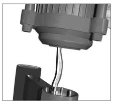
Install fixture assembly onto round fitter matching the four (4) tension rods to holes.
