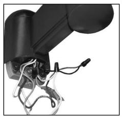
2. Mount fixture over wall mount plate. Connect fixture wires to supply wires observing polarity, i.e.; green-to-ground, white-to-common, and black-to-voltage.
