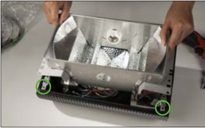
9. Pull out reflector and cut the wires connecting it to the ballast. Properly discard reflector and brackets.
