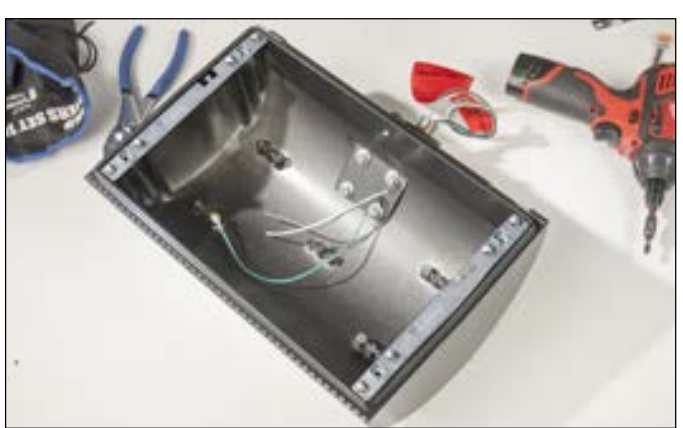
13. Secure 2 ground terminal wires to center of housing hole (1 ground ring wire from driver bracket, and 1 ground ring wire already attached to fixture). Strip white and black leads using wire strippers.
