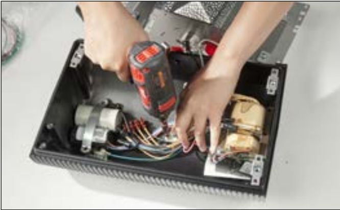
11. Using philips bit, remove: 1) Mounting strap from capacitor 2) Mounting tie from center of housing 3) Grounding wire screw
