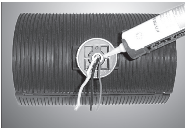
1. Apply silicone thread sealant to keep moisture out of J-Box.
