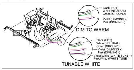
SpectraSync tunable white luminaires are provided with (2) 0-10V circuits. The violet and pink circuit is for wiring to any qualified 0-10V controller for dimming. The violet/white and pink/white circuit is for wiring to any qualified 0-10V controller for tunable white CCT control.
