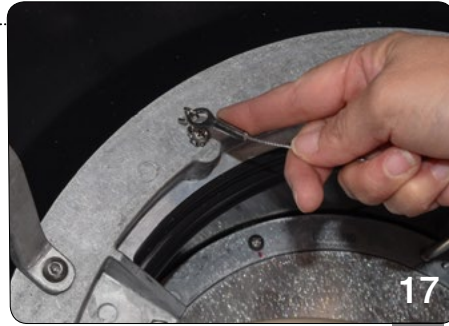
Attach (2) safety cables from new Deck Assembly. As shown.
