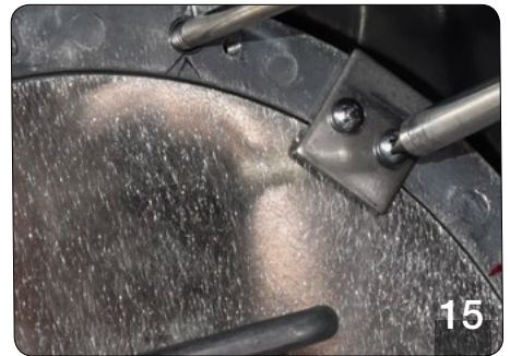
15 Secure new driver assembly back in place using existing screws/plates, secure in place (hand tighten).
