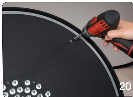
Using new 1/4-20 Screws and O-rings, attach new deck assembly to housing. Torque screws to 48 in lbs.
