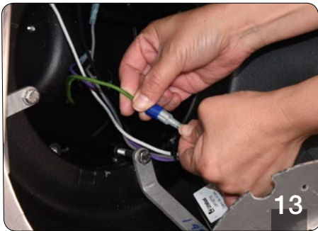
13 Connect wires from new driver assembly. Make sure to follow polarity i.e. green to green, white to white etc. Tuck leads into driver housing (make sure not to pinch wires).
