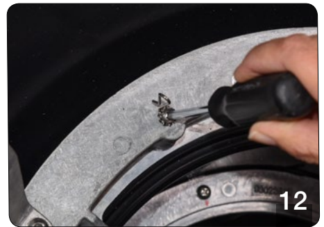
12 Install provided safety clips (2) on fixture ring As shown.
