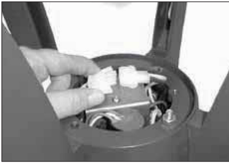
13. Disconnect wiring connectors in top of hub.
