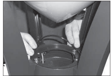
24. Install o-ring on top of retaining ring.
