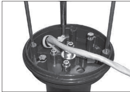
17. Remove plastic strain relief and attach supplied green ground wire in its place.
