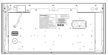
Product Label is placed near access plate as shown above according to regulatory requirements, electrical enclosure size may vary by options.
