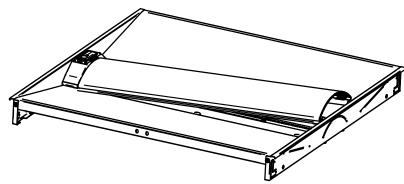
Lens can be installed into a fixture having an optional integrated sensor by first inserting end under holder, squeezing the width to snap into place against housing tabs. Ensure the lens is fully seated into place along the remaining length under housing tabs.
