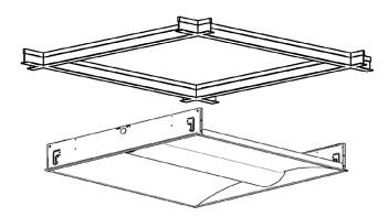
2 Install the unit into reserved space in the ceiling grid (recessed installation shown here).
