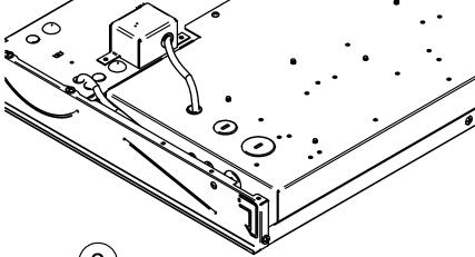
EM option test switch wiring connections are fully enclosed with plenum rated wiring or sleeving as illustrated above. EM Test Switch wiring or enclosure is not field serviceable or accessible.
