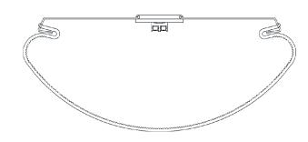
Bend the 4 clips (T-grid hooks) to secure the luminaire in place. Secure fixture to facility structure per local Building Codes. Safety cable installs through the endcap as illustrated.
