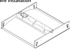
Carefully unpack unit from its packaging. Properly inspect for defects before installing. Wear work gloves to prevent dirt and oil from being transferred to the luminaire.
