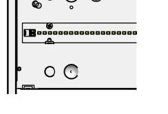
EM option having integrated battery installed will have the test switch (TS) mounted onto housing and accessible as shown. Lens must be removed to test EM switch function (not applicable for surface mounting option with side mounted TS.)
