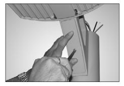
**3.** Install arm access cover and secure with self retained screw using a B" Allen wrench. Be sure wires are not pinched as screw is tightened.
