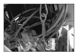
**7.** When driver tray is opened, make sure retention cable is securely attached before closing.
