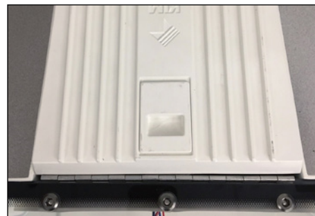
6. Align driver tray on hinge and close, pressing down until latch snaps into place.
