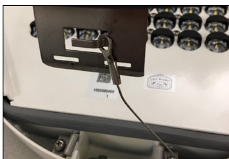
10. If a lens is present in existing housing, ensure retention cable is assembled before closing lens.
