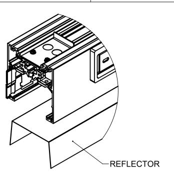
REMOVE REFLECTOR FROM ALL FIXTURES BEING MOUNTED. DO NOT REMOVE REFLECTORS FORM PROTECTIVE SLEEVE UNTIL YOU ARE READY TO REINSTALL.
