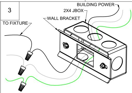
FEED WIRES FROM BUILDING POWER INTO 2X4 JBOX AND CONNECT TO FIXTURE WIRING. BRING ALL CONNECTIONS INTO FIXTURE.
