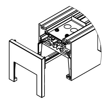
WITH RELECTOR REMOVED, REMOVE THE TWO END CAP SCREWS FROM INSIDE THE FIXTURE.PULL END CAP AWAY FROM FIXTURE. TO REINSTALL, HOLD ENDCAP TIGHT TO FIXTURE AND SCREW BACK IN.
