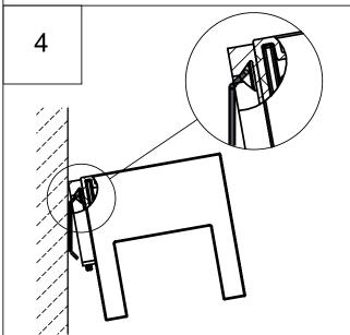
MOUNT FIXTURE ONTO BRACKETS AT AN ANGLE. ALLOW FIXTURE TO BECOME FLUSH WITH WALL SURFACE.
