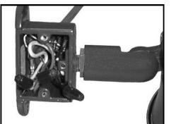
5. Make wire connections observing polarity, i.e., greentoground, white-to-common and black-to-voltage.
