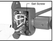
**6.** Adjust fixture and secure with set screw.
