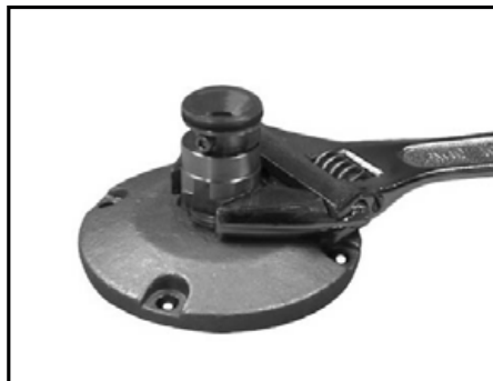
2. Tighten coupling onto mounting device. (Consult KIM Landscape Catalog for mounting device options.)
