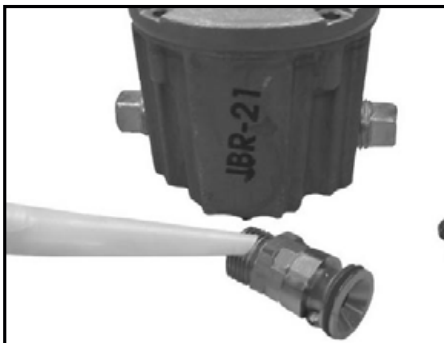
1. Coat threads with sealant to keep moisture from entering J-Box.
