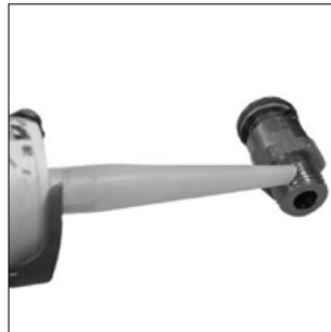
1. Coat threads with a good sealant.
