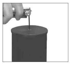
1. Remove pole cap assembly from slipfitter using 3/32" allen wrench.
