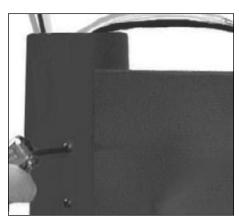
6. Using 3/16" allen wrench, secure slipfitter to tenon with four set screws (provided).
