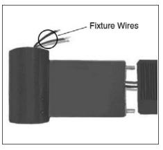
3. Feed fixture wires through arm and out top of slipfitter. Mount fixture to arm using washers and thin jam nuts, torqued to 15-20 ft.-lbs. Secure with thick nuts over jam nuts.
