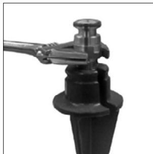
2. Tighten coupling onto mounting device.
