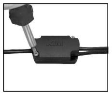
5. Attach branch connector top with the two self-tapping stainless steel Philip head screws. (provided).
