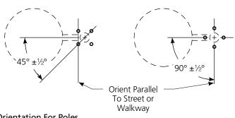
Orientation For Poles with Anchor Bolts In Corners of Base Plate.
