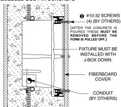
**IMPORTANT:** After concrete has been poured, the four mounting screws - • must be removed before the form is pulled off. The tapped holes in the fixture housing are used for holding the door frame assembly, the threads will be damaged if the form is forced off before the screws are removed.
