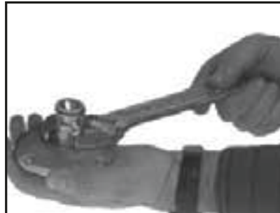
Step 2 - Tighten coupling onto mounting device*.
