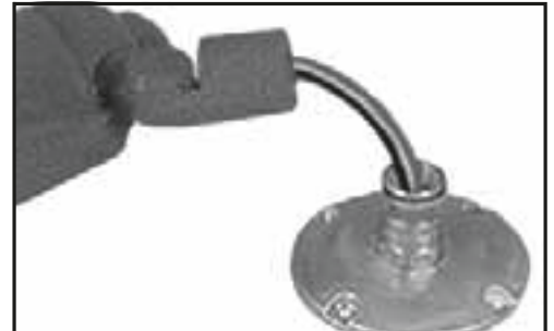
Step 3 - Install fixture onto coupling. Attach fixture leads observing polar-ity, i.e., braided bare copper wire-to-ground, white-to-common, and black-to-voltage.
