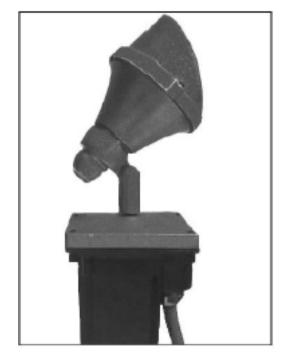
4. Make certain all grounding leads are connected to the incoming ground circuit. Make wiring connections as per wiring label in ballast compartment. Clean gasket and gasket surface. Coat cover screw threads with silicone grease and install cover.
