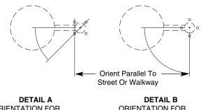
ORIENTATION FOR POLES WITH ANCHOR BOLTS IN CORNERS OF BASE PLATE
