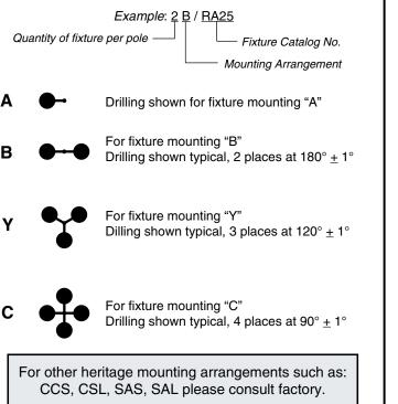
**Note:** For proper drilling of poles be sure to note fixture orientation to anchor bolts. Select one of the orientations suited to your pole and keep consistent for all poles the same. Drawings below show proper orientation for fixture mounting arrangement "A". Arrangements "B", "Y", and "C" are typical.
