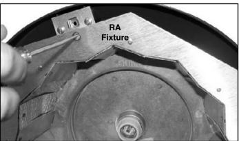
4. Secure reflector with 1/4" turn fastener. NOTE: Type 5 reflectors mount in one position.
