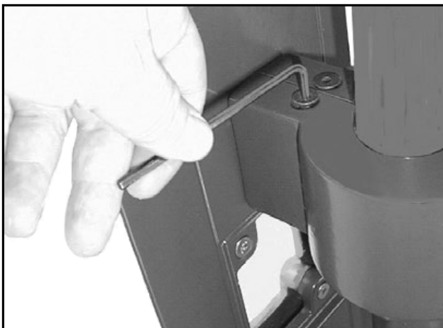
13. Install crook arm support covers and secure with center screws. ( \frac{5}{32} " Ball end "L" hex wrench recommended.)
